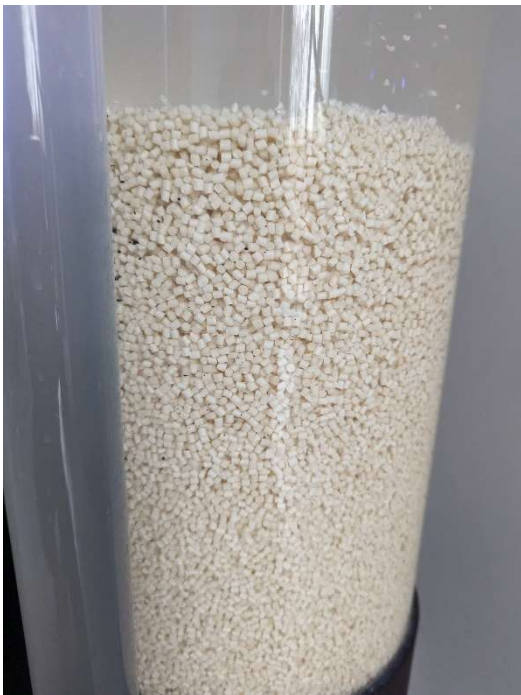
Fig. 2: Filled Pellet Filter in operation. The pellets are only whirled up slightly.
